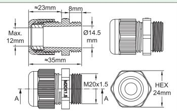
The reduced length of the thread makes it possible to mount it on enclosures with thin walls, without too much encroaching on the interior space. It has an O-ring to ensure the tightness with the enclosure, and the compression nut is self-locking. It allows to pass cable diameters up to 12mm. Made in PA6 UL94V2. Gaskets are available in 65 shore silicone or NBR 70 shore.
